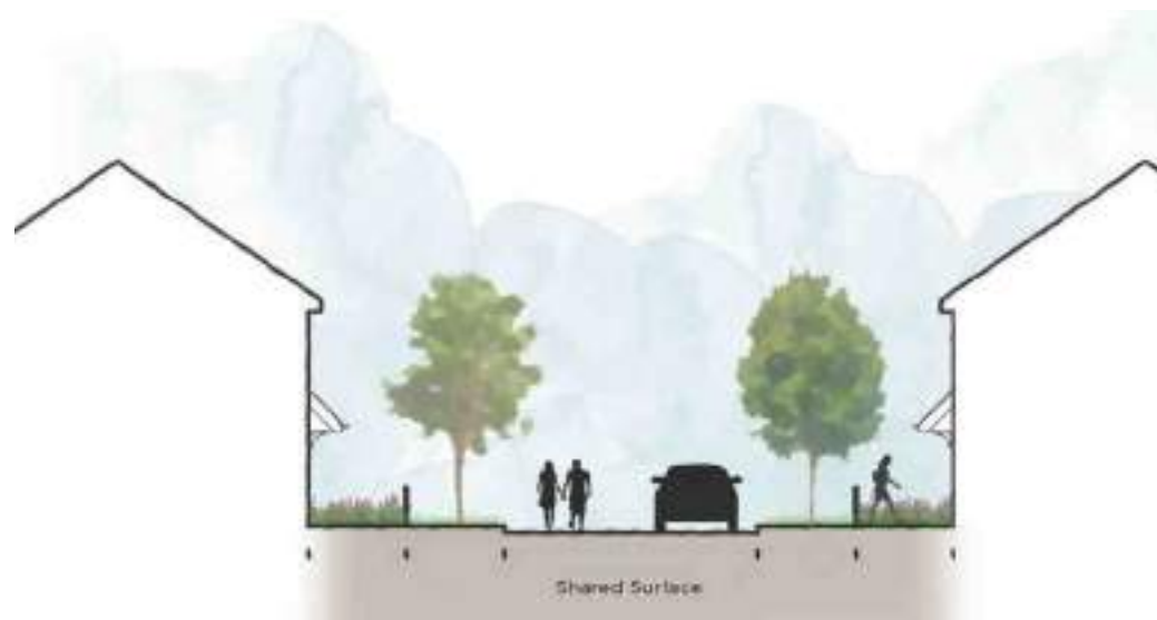
Figure 5.2.5: Shared Surface Street Section
