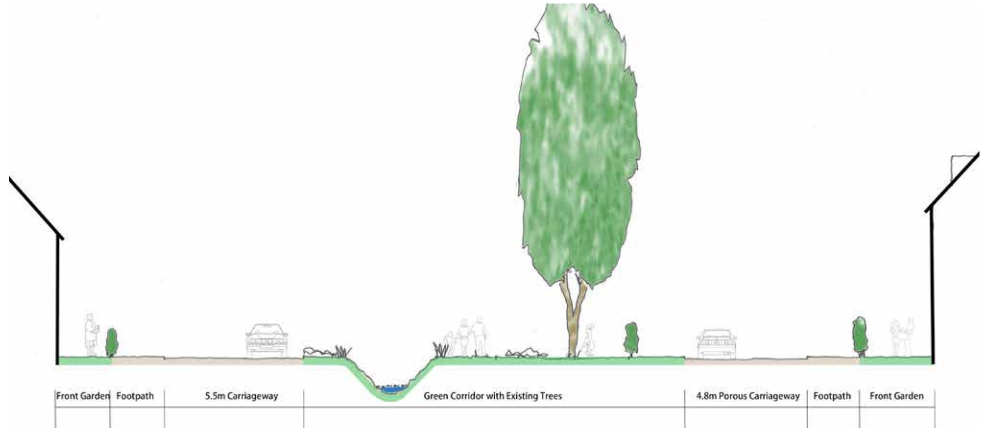
Fig 37: Street Section DD - Green Corridor
